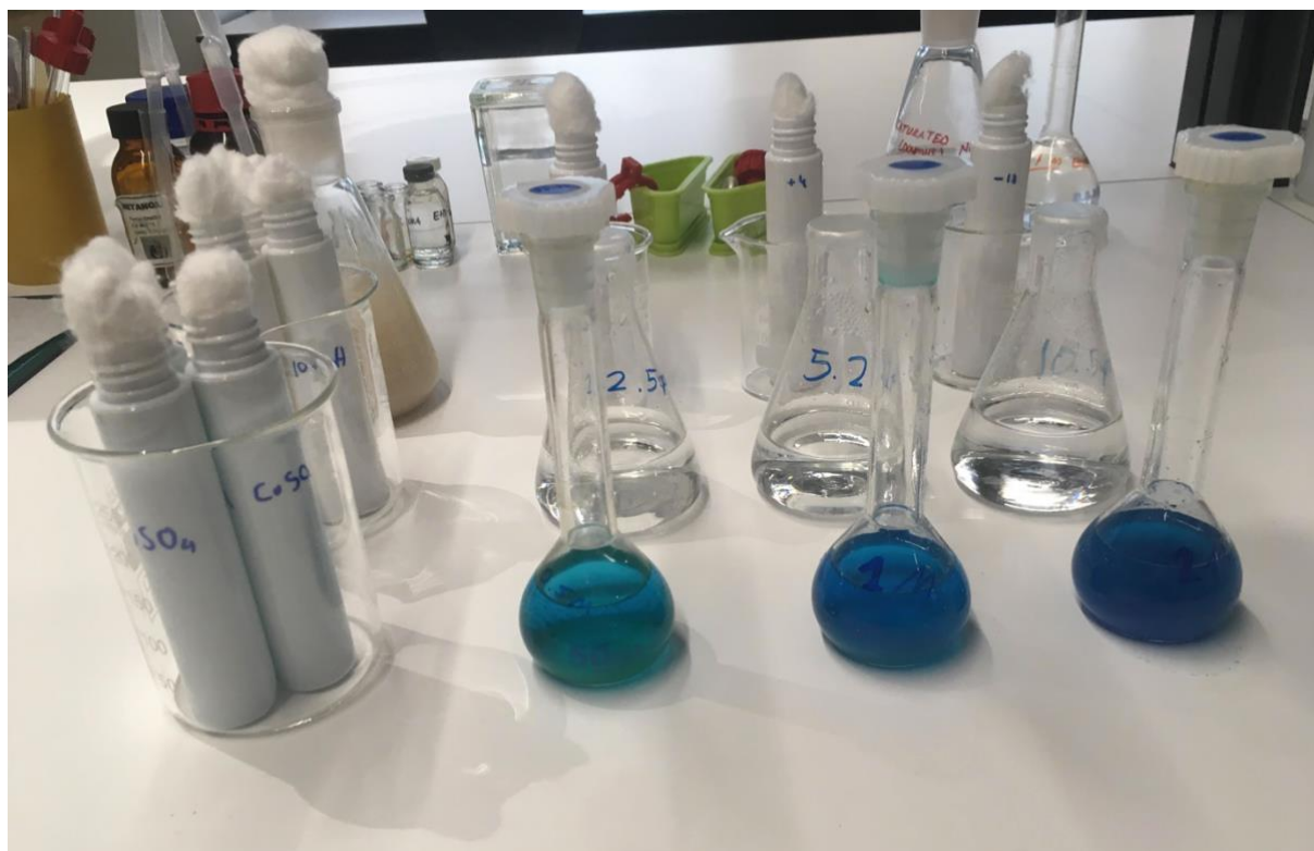
Figure 2 Experiment groups (white cylinder with cotton attached, pH stress agents (middle line) and heavy metal stress agents in different concentrations (volumetric flasks with blue solutions)
